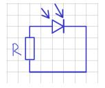
The photo diode can be used as a generator of the current. In this case the photo diode form the current. A value of the current depends on the length of light wave and a light power. Typical values are  $\sim 0.5A/W$  as  $\lambda \sim 850$  nm.
