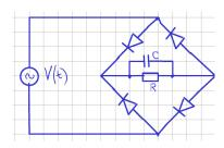
Assume  $v(t) = A \sin(\omega t)$ . In general case  $\omega = 2\pi 50 \text{rad/sec.}$ . Then the ripple frequency is about 314rad/s..
