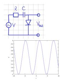
This circuit uses to get a waveform to a fixed DC value.
