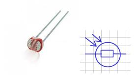
The simplest component which uses a semi-conducting property is a photo resistor or Light Dependent Resistor (LDR). The photo resistor has follow properties:
