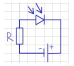
The photo diode can be considered as a photo detector. In this case the diode connect as a reverse bias. The current without the light the inverse current is about  $\mu A$ , but the current with the light is about 10mA.
