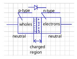
A np-junction forms internal voltage without an external electric field. This voltage jump appears because of motion the wholes to the n-doped piece of the diode. The opposite side forms by the electrons which dissipates into the p-doped part of the junction. Near the border a layer
